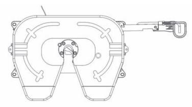
Figure 8 - Fifth wheel in Open position
