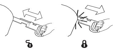
Figure 6 - Locking of a fifth wheel with an Interlock handle
