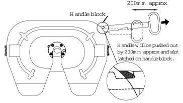
Figure 3 - Fifth wheel in Open position
