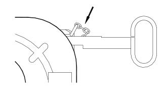
Figure 5 - Locking of a fifth wheel with a Standard handle
