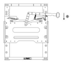
Figure 4 - Slider in open position ready for adjustment
