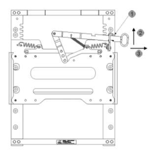
Figure 3 - Slider in locked/closed position ready for operation
