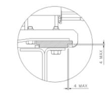
Figure 8 - Wear limits for outer guides
