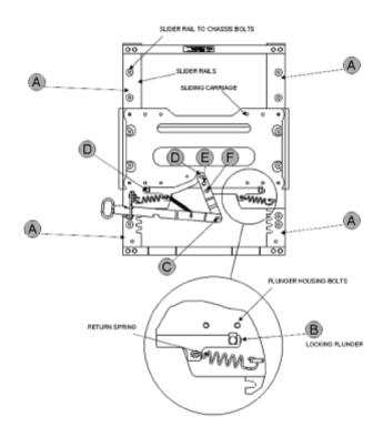
Figure 7 - Labelled slider carriage
