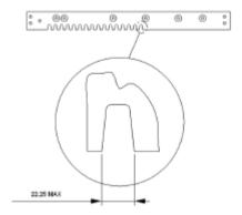
Figure 12 - Slider rail dimension limits
